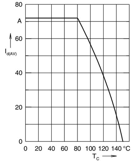
Fig. 5 Max. forward current versus case temperature
