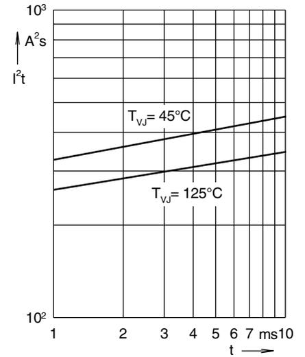
Fig. 3 I<sup>2</sup>t versus time per diode
