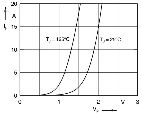
Fig. 20 Typ. forward characteristics of free wheeling diode
