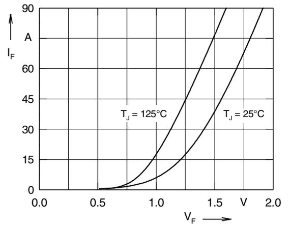
Fig. 10 Typ. forward characteristics of free wheeling diode
